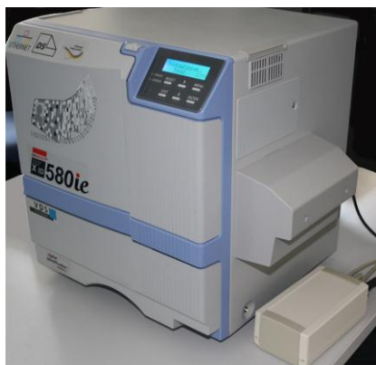
EDIsecure ® XID 580ie Retransfer Printer with 'RFID Encoder Box' (to the right)
